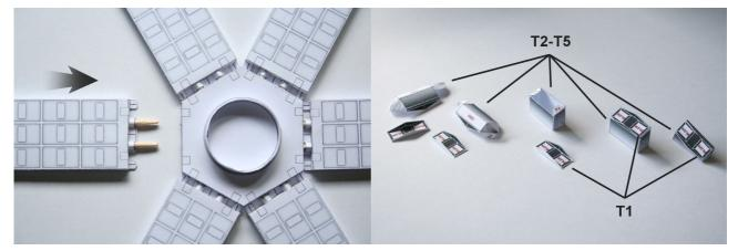
Push the toothpicks of the LAD-panels into the holes of the Optical Bench, and fix them with glue. Form five support trusses from parts T1-T5 like seen above.
